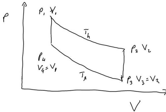
Figure 1: Find the work and efficiency of a cycle.
